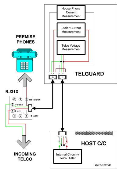
The TELGUARD has to be the first device on the incoming telco line. No telco device can be in front of or in parallel with the TELGUARD or a Line Fault condition will occur.
